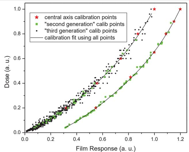
**Figure 2:** The figure displays the primary, secondary, and tertiary calibration points along with the fit that generates the film calibration curve for a five 15mm cone pattern. A second set of primary and secondary calibration points along with the film calibration curve is displayed shifted by 0.2, generated from six 10mm cone pattern. Both axes have arbitrary units.
