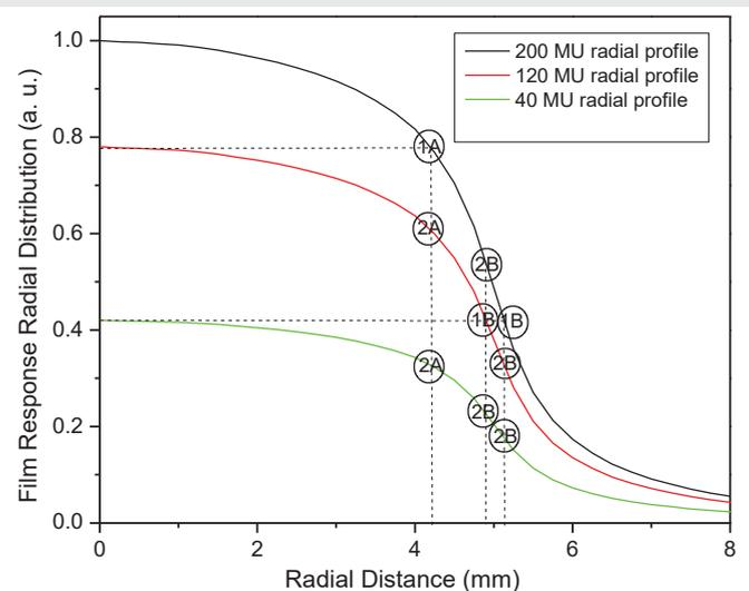
**Figure 1:** The figure displays three of the five film response radial profiles for the 10 mm cone for 200MU (black), 120MU (red), and 40MU (green) and describes the method for generating "secondary calibration points".
